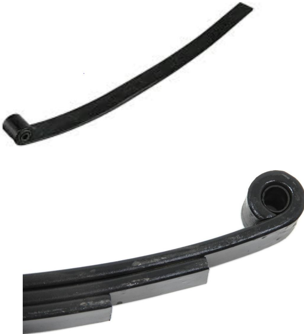
Examples of single and triple leaf springs.
